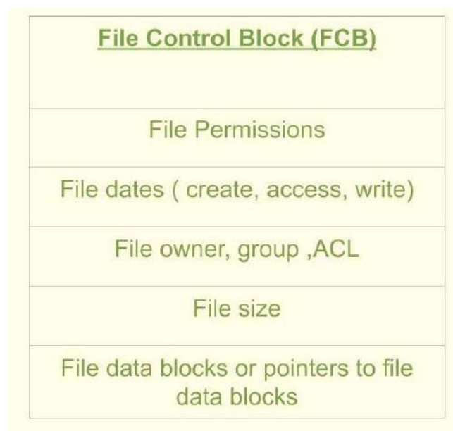
Structure of File Control Block (FCB)
